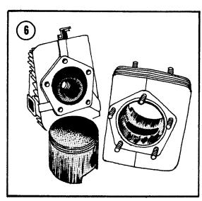
3. If compression is low or variance between cylinders is excessive, check for defective head gaskets, damaged cylinders and pistons, or stuck piston rings.
