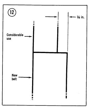
actuation or rough or scratched pulley surfaces. If all mechanical systems are functioning properly, the belt may just be worn out. Replace drive belt if its width is ¼ in. (3mm) less than new. Refer to Chapter Seven.
