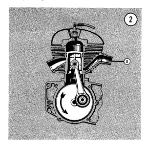
The third phase is shown in Figure 3. As the piston approaches top dead center, the spark plug fires, igniting the compressed mixture. The piston is then driven downward by the expanding gases.
